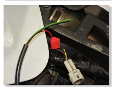
CUT THE YELLOW WIRE. CONNECT THE BLP RED WIRE TO YELLOW WIRE END, WHICH IS AT THE WIRING HARNESS SIDE.
