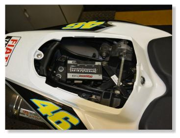
LOCATE THE REAR LIGHT CONNECTOR BETWEEN PASSANGER AND MAIN SEAT. (WHITE, 3-POLE TRIANGULAR CONNECTOR)
