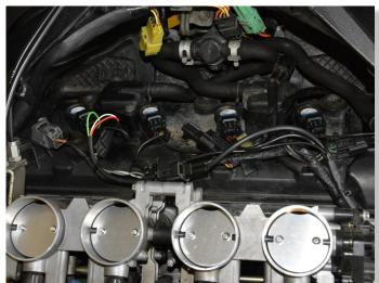
MOUNT THE QSX MODULE TO THE INNER SIDE OF THE FRAME WITH THE SUPPLIED VELCRO STRIPS, AND SECURE THE CABLES WITH CABLE TIES.
