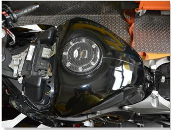
LIFT UP OR REMOVE THE FUEL TANK.
