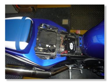
LIFT UP OR REMOVE THE FUEL TANK.
