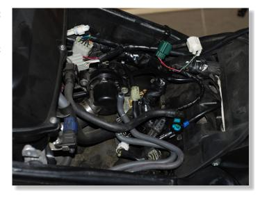
PLUG THE GPX CONNECTORS IN-LINE WITH THE SPEED SENSOR CONNECTORS.
