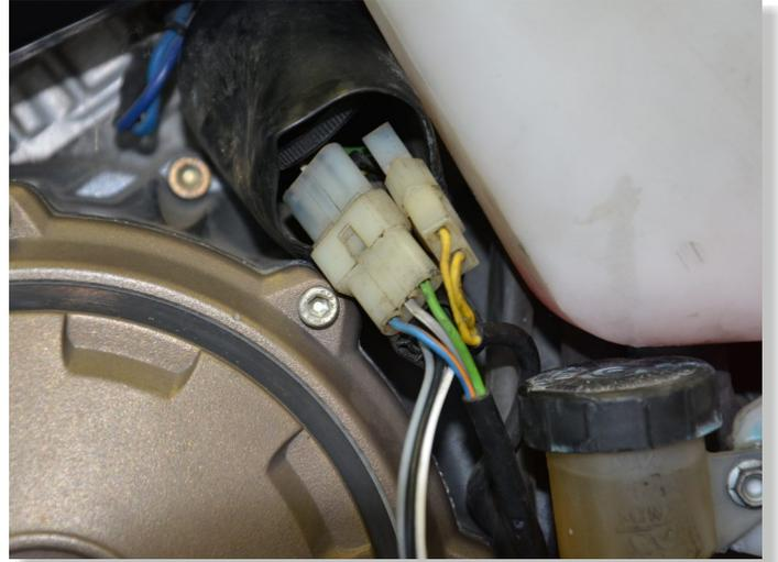
**CONNECT GPX RED WIRE TO RED WIRE OF SPEED SENSOR CONNECTOR.**
