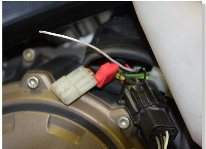
**CONNECT GPX WHITE WIRE TO GRAY/WHITE WIRE OF SPEED SENSOR CONNECTOR.**
