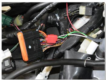
CONNECT GPX RED WIRE TO RED/WHITE WIRE OF ECU/ECM CONNECTOR.
