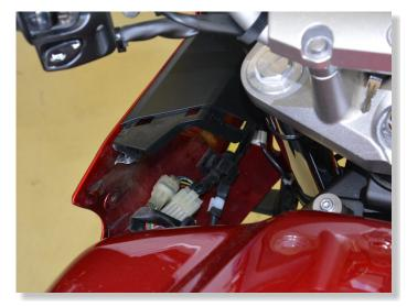
REMOVE THE SEAT. LIFT UP OR REMOVE THE FUEL TANK.
