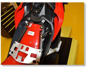
LOCATE THE REAR LIGHT ASSEMBLY CONNECTOR. (Black, 3-pole connector, next to the diagnostic port)
