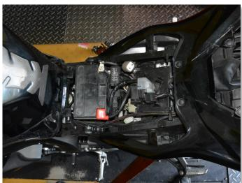
LIFT UP OR REMOVE THE FUEL TANK.
