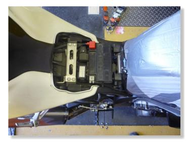
LIFT UP OR REMOVE THE FUEL TANK.
