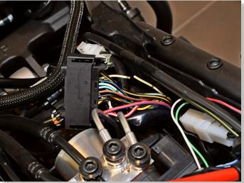
Splice the SpeedoHealer white wire to the white/yellow wire end, which goes to the ABS ECU connector.
