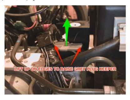
Remove the protective cap from the plug, exposing the wires coming out of it. A small screwdriver can be carefully used to un-do the 4 snaps securing this cap. Carefully fan out the wires.
