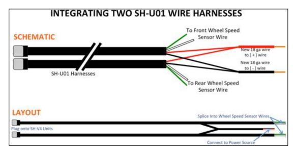
At the ABS plug, cut the **White/Yellow wire for the Rear Wheel** Speed about 4-5 cm from where it goes into the black wrapped wiring harness. You must have enough of the wire free to stick it ALL the way into the 3M Scotchlok UY2 connector and not have a sharp bend or kink in the wire.
