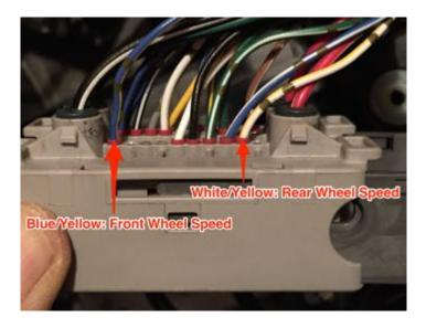
The Rear Wheel Speed wire is White and Yellow (W/Y). Front Wheel Speed wire is Blue and Yellow (L/Y). Installing SH on the REAR wheel circuit is REQUIRED, adding a second SH to the FRONT is optional (see note on page 1).
