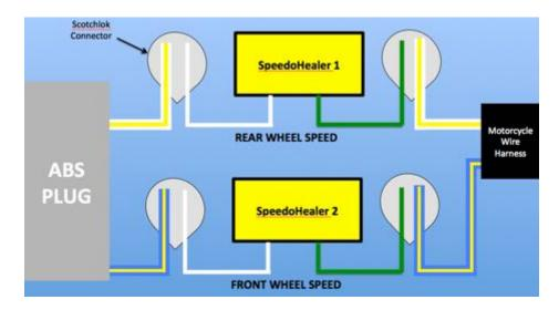
Insert the WHITE/YELLOW wire **from the ABS plug** into one of the holes in the 3M Scotchlock connector, and the WHITE wire of the SH into the other. Make sure both wires are pushed ALL the way in, then carefully squeeze the orange button into the connector. Try to press it STRAIGHT in. You may see some gel inside the connector – this is for waterproofing the connection.
