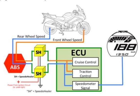
The Engine Control Unit ("ECU") does not add the extra amount to the odometer. Installing SpeedoHealer(s) will likely alter your odometer accuracy. In some jurisdictions this is against the law. Check your local laws and do not install SH if is illegal. It may also affect the warranty and/or the re-sale value of the motorcycle. This is all at your own acceptance and risk.
