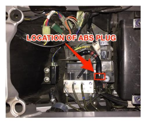
Un-plug the ABS control unit. To do this, the dark gray plastic keeper tab on top of the plug must be pulled all the way up (about 6 cm). DO NOT pull on any of the wires. Pull only on the plastic keeper structure itself. Pulling that keeper extracts the plug straight out from the socket. Once you have pulled the grey keeper out, the plug is free.
