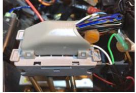
Rear Wheel Speed Sensor spliced in, and with the wire protector cap back on. The Front Wheel Speed splice is not shown in this photo.
