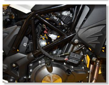
UNPLUG THE ABS ECU CONNECTOR. (Black, 18 pole connector under the fuel tank, Next to the ABS unit.)
