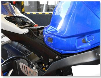
LIFT UP OR REMOVE THE FUEL TANK.
