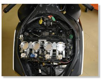
PLUG QSH CONNECTORS IN-LINE WITH THE IGNITION COIL CONNECTORS. (BLACK, 2-POLE CONNECTORS BELOW AIRBOX)
