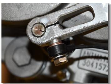
TIGHTEN THE BOLT IN THIS POSITION BY 6 NM USING A TORQUE WRENCH.
