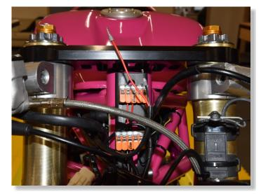
MOUNT THE IQSE-2 UNIT WITH THE SUPPLIED VELCRO STRIP UNDER THE FRAME NECK.
