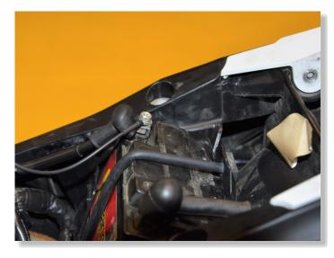
USE THE ORIGINAL BOLT OF THE GEARBOX SHAFT, ADD THE SENSOR AND THE ORIGINAL WASHER EXACTLY AS SHOWN IN THIS PHOTO.
