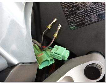
RELEASE AND REMOVE THE GREEN/RED AND BLACK WIRES FROM FEMALE CONNECTOR. (GREEN, 4-POLE CONNECTOR AT LEFT SIDE BELOW MIDDLE FAIRING)
