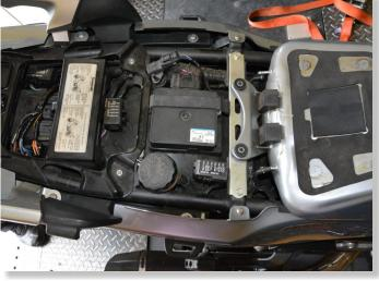
LOCATE THE GPS (GEAR POSITION SENSOR) COUPLER. (GREEN, 4-POLE CONNECTOR AT LEFT SIDE BELOW MIDDLE FAIRING)
