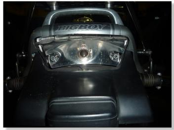
CONNECT THE BLP RED WIRE TO GREEN/YELLOW WIRE OF REAR LIGHT CONNECTOR, WHICH IS AT THE WIRING HARNESS SIDE.
