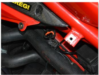
CONNECT QSH CONNECTORS IN-LINE WITH THE IGNITION COIL CONNECTOR OF REAR CYLINDER.
