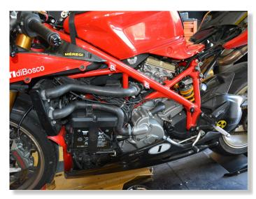
CONNECT QSH CONNECTORS IN-LINE WITH THE IGNITION COIL CONNECTOR OF FRONT CYLINDER.
