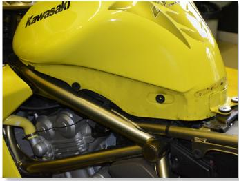
LIFT UP OR REMOVE THE FUEL TANK.
