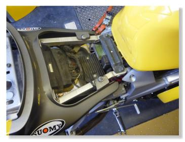
LIFT UP OR REMOVE THE FUEL TANK.
