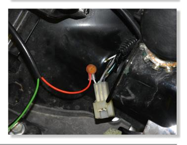
CONNECT THE BLP GREEN WIRE TO WHITE/BLACK WIRE END, WHICH IS AT THE WIRING HARNESS SIDE.
