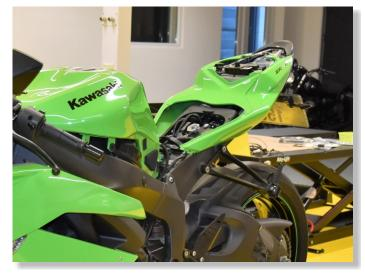
REMOVE OR LIFT UP THE FUEL TANK.
