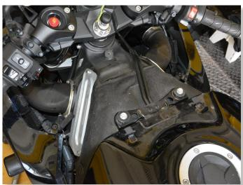
CONNECT QSH CONNECTORS IN-LINE WITH THE IGNITION COIL CONNECTORS.
