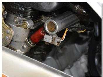
CONNECT QSH CONNECTORS IN-LINE WITH THE INJECTORS AND INJECTOR CONNECTORS.
