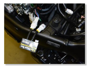
MOUNT THE X-TRE BOX TO THE INNER SIDE OF THE FRAME BY THE SUPPLIED VELCRO STRIPS, AND SECURE THE BOX AND CABLES WITH CABLE TIES.
