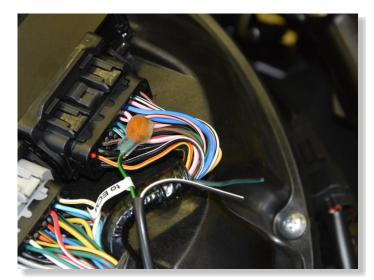
CONNECT THE X-TRE BLACK/WHITE WIRE TO BLACK/GREEN WIRE END, WHICH IS AT THE WIRING HARNESS
