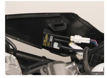
MOUNT THE X-TRE BOX TO THE INNER SIDE OF THE SIDE FAIRING BY THE SUPPLIED VELCRO STRIPS, AND SECURE THE BOX AND CABLES WITH CABLE TIES.
