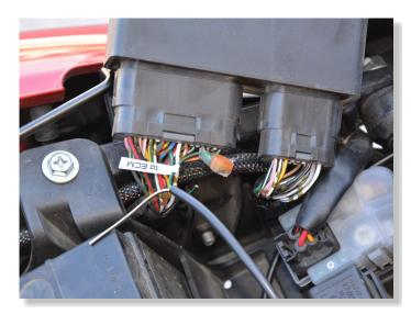
CONNECT THE X-TRE BLACK/WHITE WIRE TO BLACK/GREEN WIRE END, WHICH IS AT THE WIRING HARNESS
