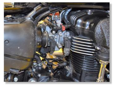
PLUG THE STVE MODULE INTO THE WIRING HARNESS CONNECTORS.
