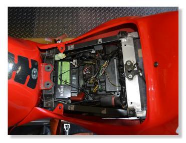
LIFT UP OR REMOVE THE FUEL TANK.
