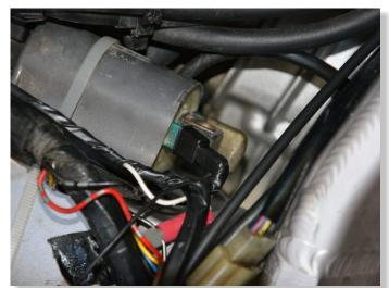
SPLICE THE QSH WHITE WIRE TO THE BLACK/WHITE WIRE OF CRANKSHAFT POSITION SENSOR CONNECTOR BY USING THE SUPPLIED RED WIRE TAP CONNECTOR.
