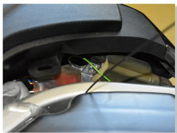
SPLICE THE QSH WHITE WIRE TO THE YELLOW/BLUE OR BLUE/YELLOW WIRE OF THE COIL BY USING THE SUPPLIED RED WIRE TAP CONNECTOR.
