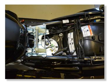
LIFT UP OR REMOVE THE FUEL TANK.
