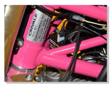
CONNECT THE 2-POLE CONNECTOR OF THE SENSOR TO THE UNIT.
