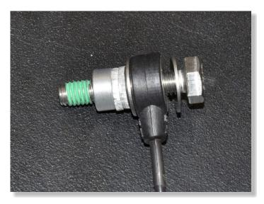
REPLACE THE BOLT OF THE SHIFT LEVER BY THE SUPPLIED BOLT AND ADD THE THICK SPACER (4,4MM), THIN SPACER (2,2MM), CONICAL WASHERS AND SENSOR EXACTLY AS SHOWN ON THIS PHOTO.
