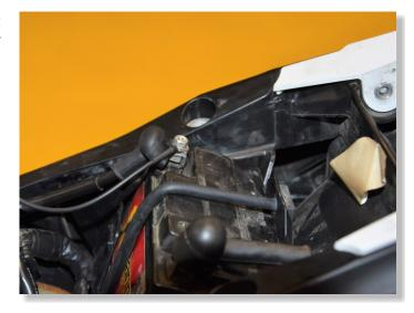
USE THE ORIGINAL BOLT OF THE GEARBOX SHAFT, ADD THE SENSOR AND THE ORIGINAL WASHER EXACTLY AS SHOWN IN THIS PHOTO.
