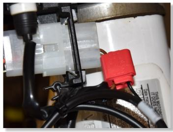
CONNECT GPX RED WIRE TO THE FI WARNING LAMP CONNECTOR ORANGE WIRE.
