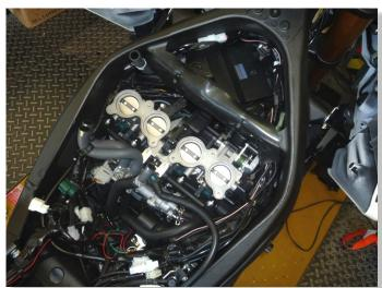
CONNECT THE GPX WIRES TO THE ECU/ECM WIRES.
