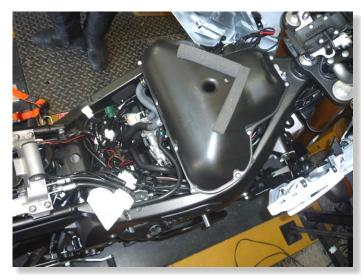
REMOVE THE AIRBOX. ECU/ECM LOCATED BELOW THE AIRBOX.
