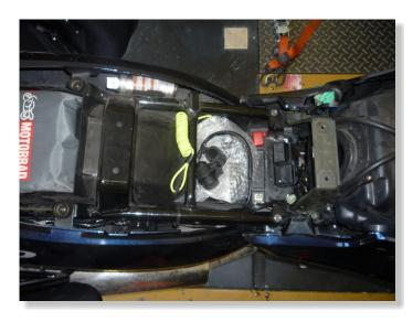
LIFT UP OR REMOVE THE FUEL TANK.
