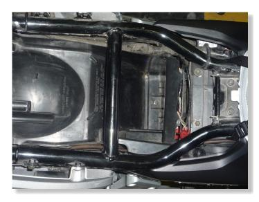
REMOVE THE LEFT AND RIGHT FRAME COVER BELOW THE SEAT.
